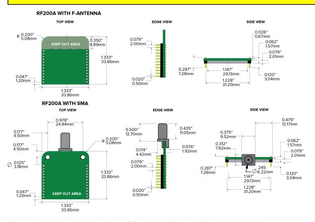
Figure 1.1: Mechanical drawings of the RF200PD1 and RF200PF1 Modules
