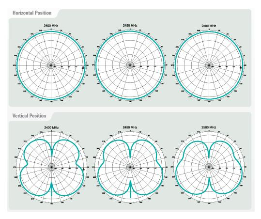
Figure 1.4: Pulse W1027 Antenna Gain Performance
