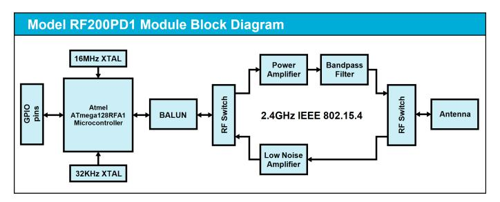
Figure 1.3: Block diagram showing the major subsystems comprising the RF200
