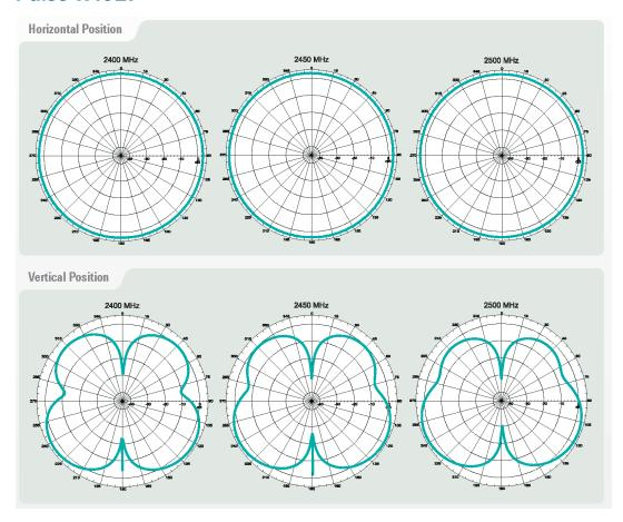
Figure 1.4: Pulse W1027 Antenna Gain Performance
