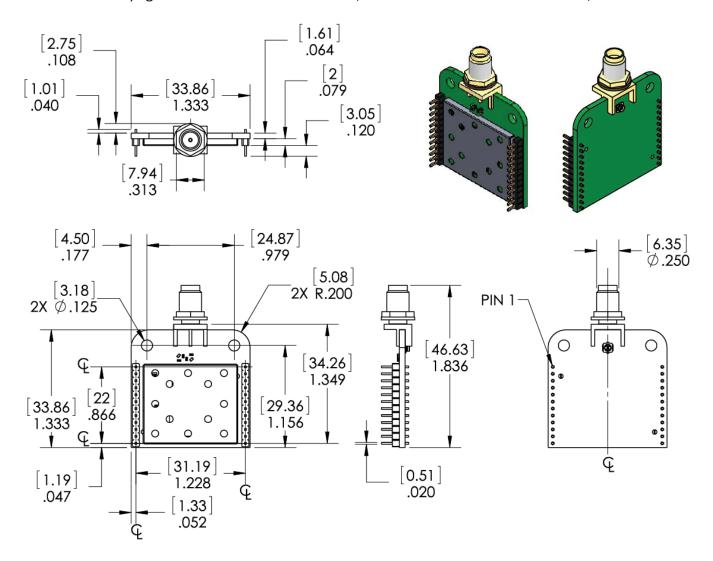
Figure 1.1: RF220SUMechanical Drawing
