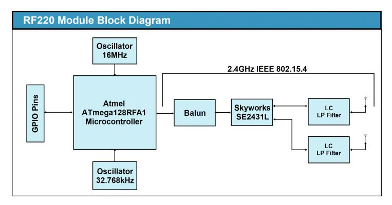
Figure 1.2: Block diagram showing the major subsystems comprising Model RF220SU
