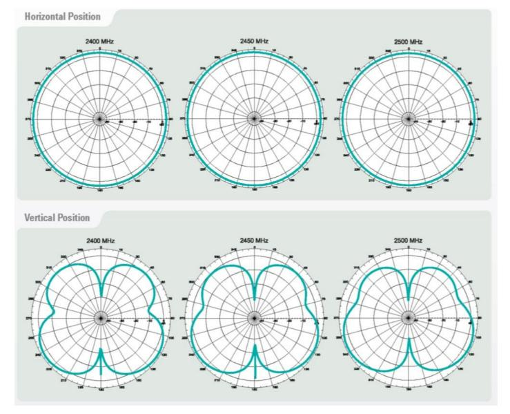
Fig. 2: Pulse W1027 Antenna Gain Performance
