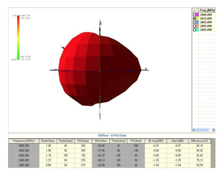
Fig. 1: Partron SDBTPTR3015 Antenna Gain Performance
