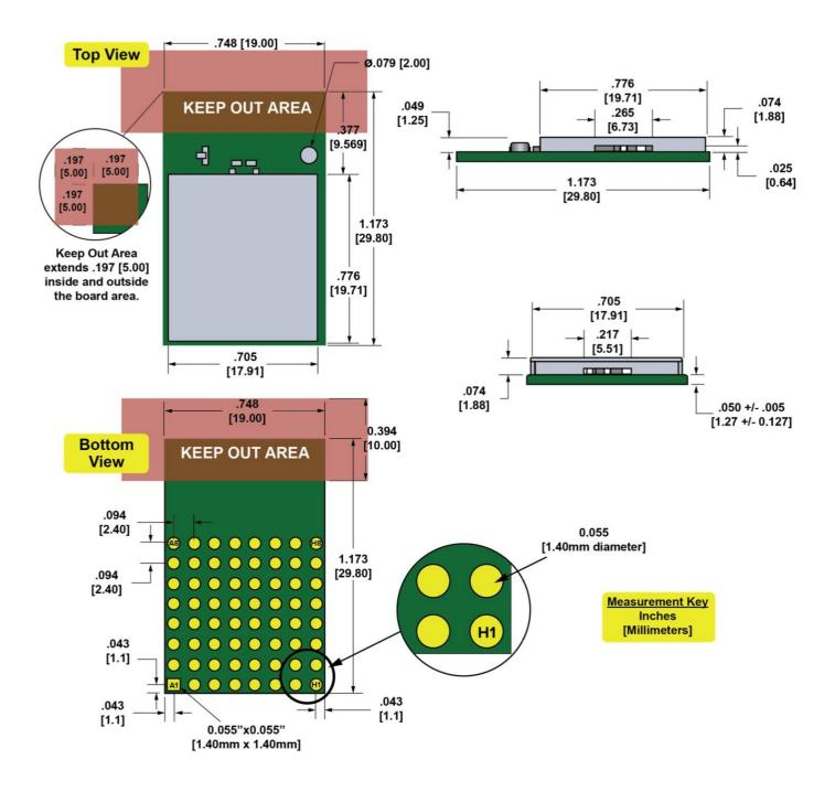
Fig. 1: SM200PF1/PU1 Mechanical Drawing
